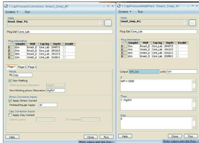
*Make pressure corrections in the main module and run calculations using the Capillary Pressure Array Mathpack.*
