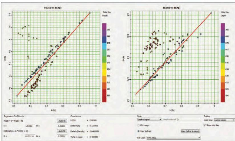
The simultaneous inversion process is stabilized by including a background relationship between P-Impedance, S-Impedance, and Density. **Strata** derives this relationship graphically using the existing wells in the project.
